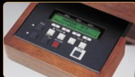
The drawbars, control tablets and rotary controls affect the operations necessary for performance on the organ. Advanced features such as drawbar voice mode, pedal sustain length etc., are accessed using the Information Center. This allows the player to see and make changes. The Information Center Display and touch buttons are located on a drawer unit positioned under the right side of the lower manual.
